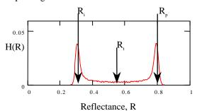
Figure 1: Histogram of 65 LPI AM halftone printed by offset lithography, measured at 5 mm field of view (FOV)
