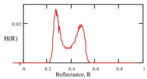
Figure 3. Histograms at 5mm FOV of error diffusion dot pattern printed by thermal ink jet at 300 dpi at a nominal F = 0.5.
